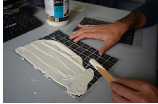
Figure 4: Example of the adversarial fingerprint physical spoof realisation. The expert is depositing a layer of latex over the printed adversarial fingerprints.
