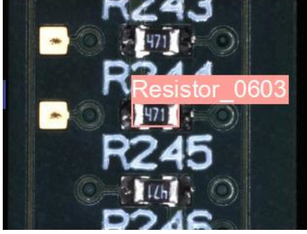
Figure 1: Example of the original 1278x958 training images we were provided: the component at the center of the image is annotated with type (Resistor) and case size (6x3 millimeters).
