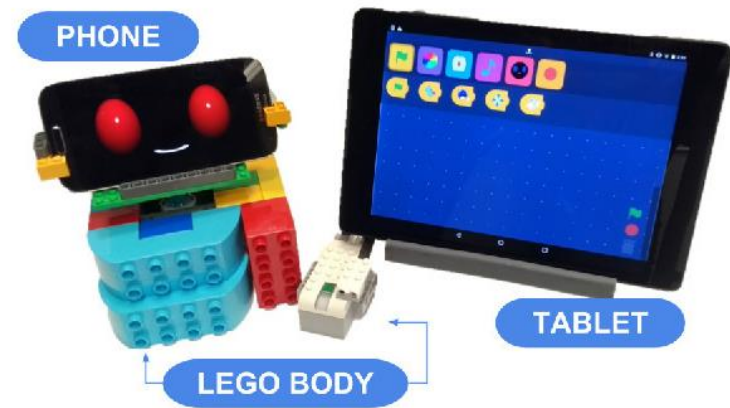
Figure 1: The PopBots platform consists of a smartphone-based social robot, LEGO blocks, LEGO WeDo motors, and a block-based programming interface on a tablet.
