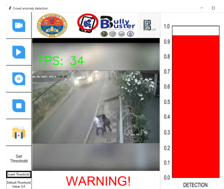
Figure 4: Demonstrator of the crowd analyzer built into the BullyBuster framework. The system detects suspicious behaviour and reports it to a human operator.
